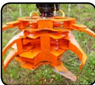
Biojack 300E grapple in an open position
